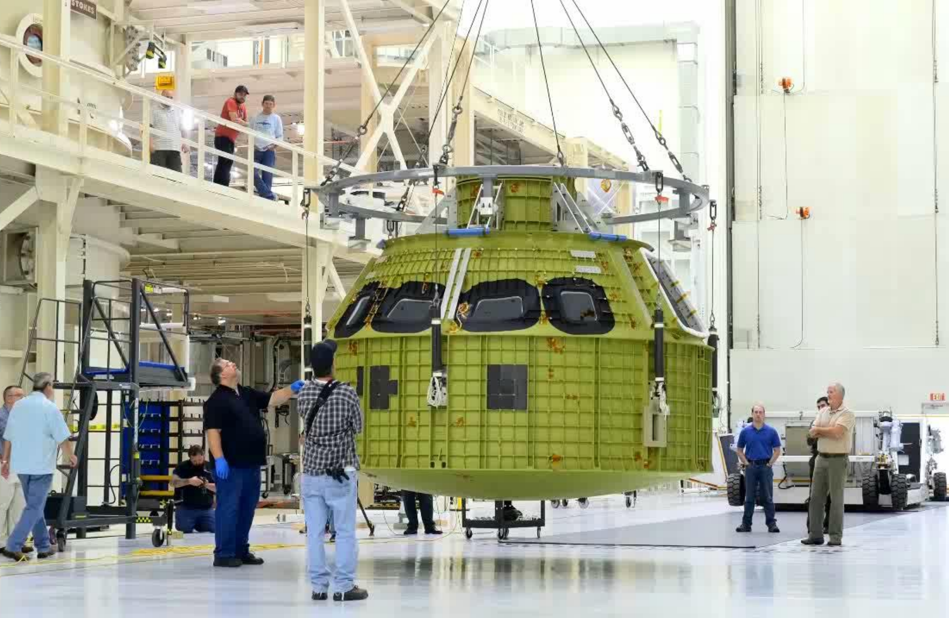
EM-1 CREW MODULE PRESSURE VESSEL OPERATIONS AND CHECKOUT BUILDING, KENNEDY SPACE CENTER, FLORIDA
