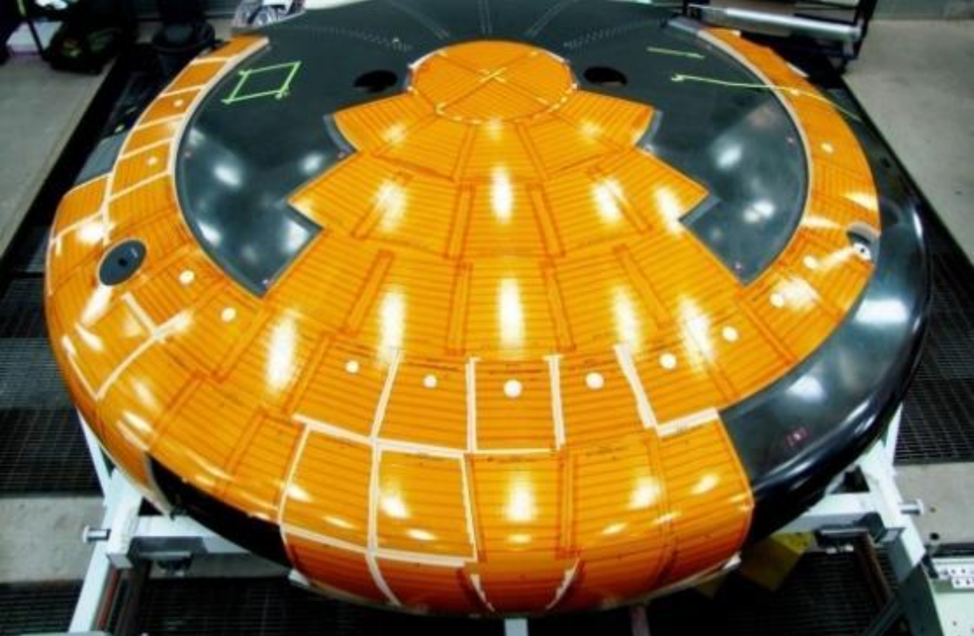
HEAT SHIELD MANUFACTURING DEVELOPMENT UNIT LOCKHEED MARTIN, LITTLETON, COLORADO
