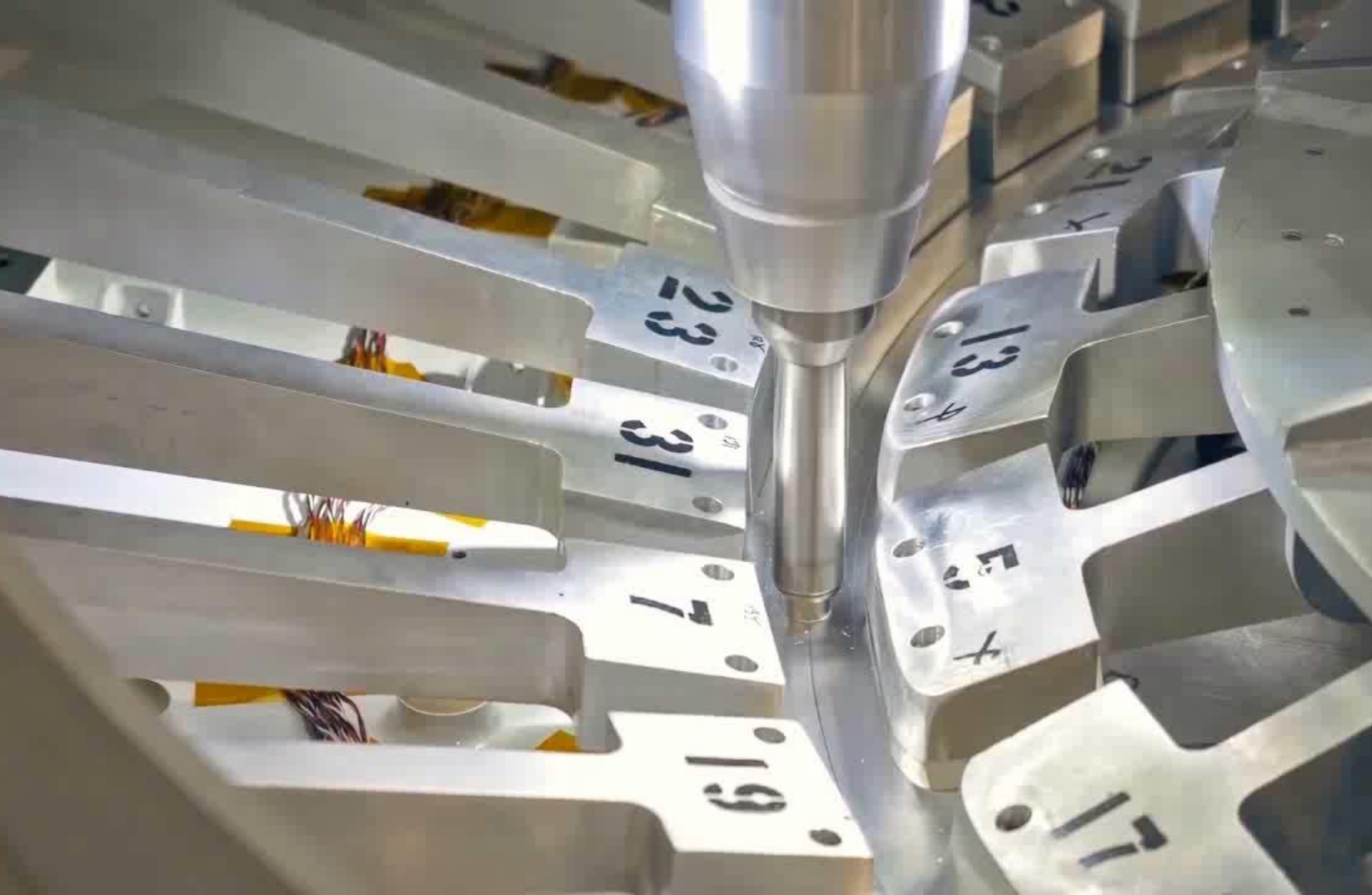
EM-1 CREW MODULE PRESSURE VESSEL WELDING MICHLOUD ASSEMBLY FACILITY, NEW ORLEANS, LOUISIANA
